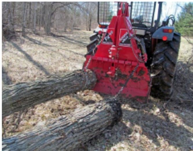
**Firewood logging with a medium sized, 4 WD tractor and winch is most common.**
